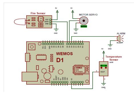
Figure 1: A prototype circuit for an early fire detection device.
